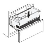
**4** Push the button and engage the stopper on either side.
