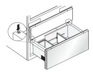
**3** Remove the basket by lifting the basket from the rail system.
