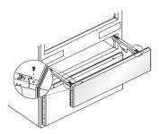
**3** Pull the drawer open to full extension Lower the basket onto the rail system.
