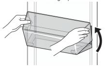
To assemble the door bin, align both sides of the bin with the guides and push the bin down until it snaps into place.
