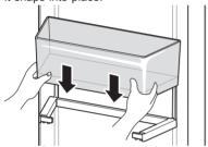
To adjust the location of the bin, tilt the front of the bin up and slide the bin up or down to the desired location.
