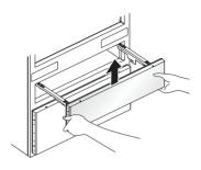
5 Hold both sides of the door and lift it to remove it from the rail system.
