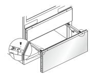
5 Hold both sides of the door and lift it to remove it from the rail system.
