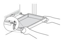
2 Keeping both levers pressed, lift the drawer support slightly and remove it from the rail system.
