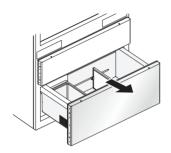
2 Push the button and disengage the stopper on either side.
