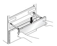
2 Insert screws at the end of both rails.
